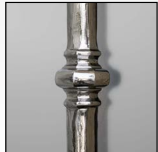
Result of the application of De-rusting and Passivating products
